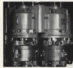
Seaming heads each contain two first and two second operation seaming rolls mounted on tapered bearings. Rolls follow the can configuration through the use of form cams.
